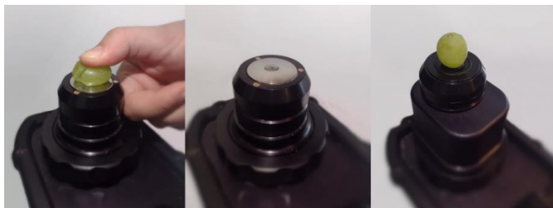
Figure S2. Illustrative photos taken during the analysis of grapes using the different configurations: a) ATR-FTIR for intact grape; b) ATR-FTIR for crushed grape; and c) DRIFT for intact grape.
