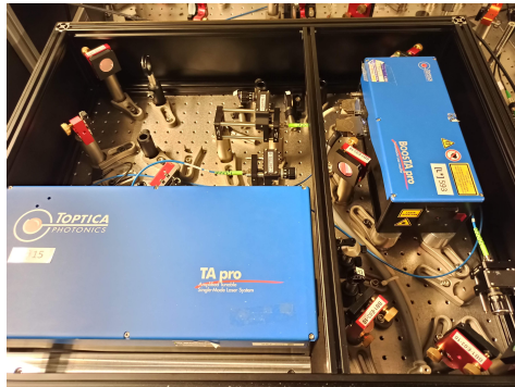
Figure B.2: Box enclosing the TA pro laser and the BoosTA pro tapered amplifier. The first PM-fiber above the TA pro serves the purpose of bringing its output to the external tapered amplifier, while the other one brings the output of the BoosTA pro to the quantum frequency conversion experiment setup.
