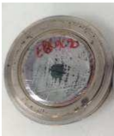
Figure 7. Sample set up for XRD analysis.
