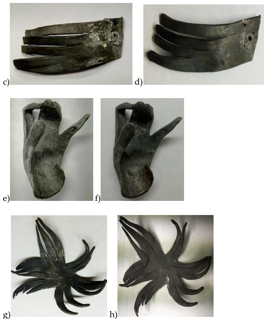
Figure 6-15. Before and after non-thermal plasma cleaning of corroded specimens, a and b ; violin handle, c and d ; hair piece, e and f ; left hand of the violinist; g and h ; hair piece.
