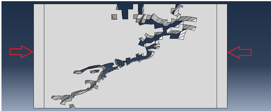
Figure 5.11: The crack path for longitudinal compression for E-glass/MY750 epoxy
