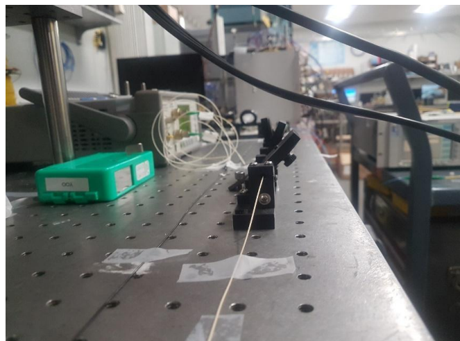
Figure 5-8- MPC configuration for D SOP
