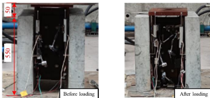
(a) General failure mode
