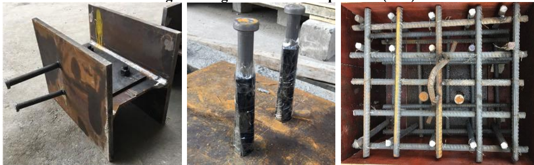
(a) steel beam assemblage (b) stud wrapped with rubber sleeves (c) rebar assemblage
