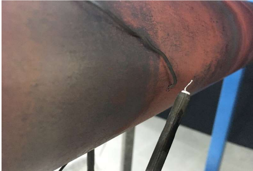
Figure 5-3. The external B and the K type thermocouples inside/outside of the pipe wall.
