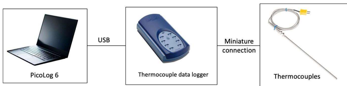
Figure 3-32. Scheme of the thermocouples and their communications interfaces with PicoLog.
