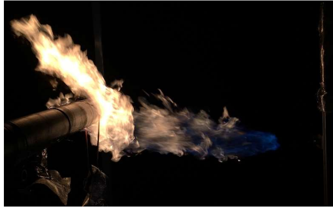
Figure 5-8. Example of impingement at the front zone.
