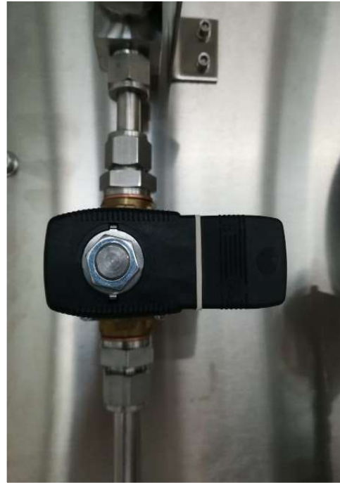
Figure 3-19. Electrical solenoid valve.
