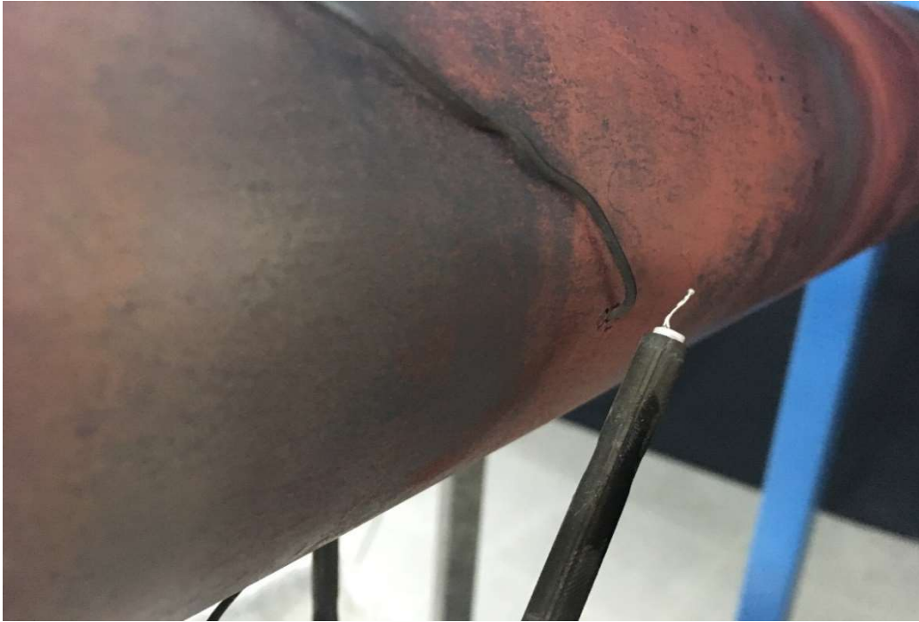
Figure 3-9. The location of the two thermocouples (inside and outside the pipe wall) at the front position.
