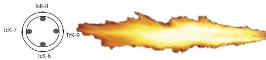
Figure 3-8. Scheme of the position of internal thermocouples.
