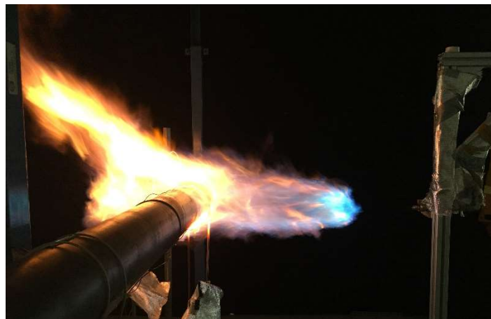
Figure 5-7. Example of impingement at the middle zone.
