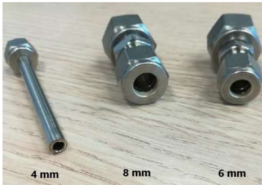
Figure 3-25. Gas release nozzles.
