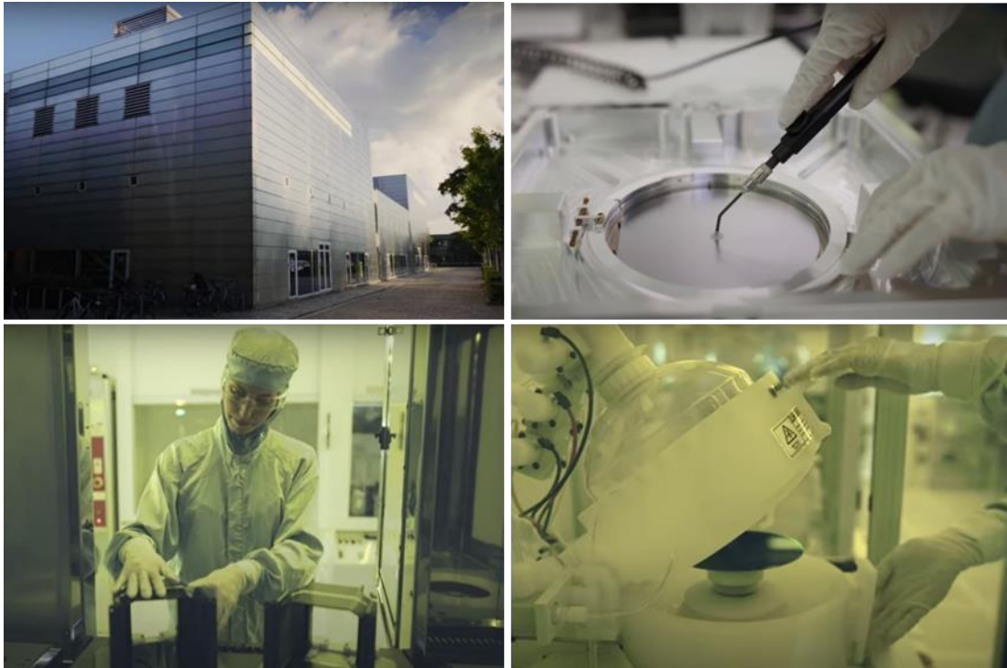
Figure 3.1. Images of the DTU Nanolab cleanroom facilities: (top left) the cleanroom building; (top right) electron beam lithography cassette loading; (bottom left) automatic resist spin coaters; (bottom right) automatic electron beam resist developer.
