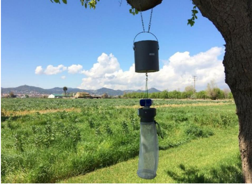
Fig 1. Classic EVS mosquito trap baited with a container with CO 2 pellets.
