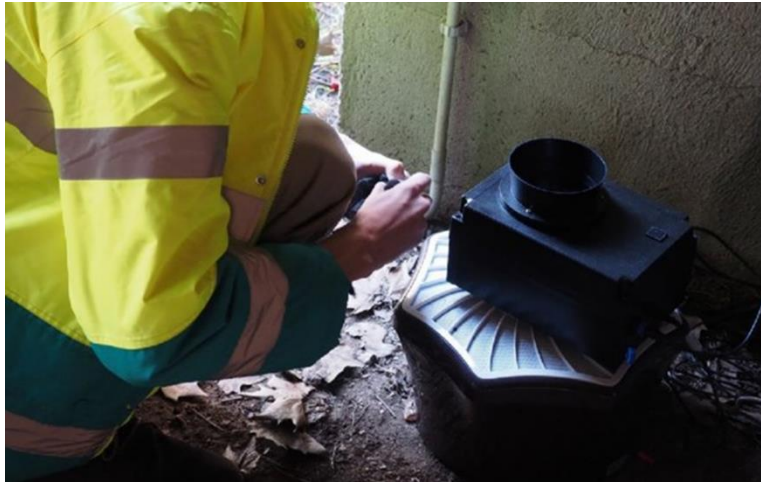
Fig 3. Vector control technician installing a trap with IRIDEON's smart mosquito sensor.
