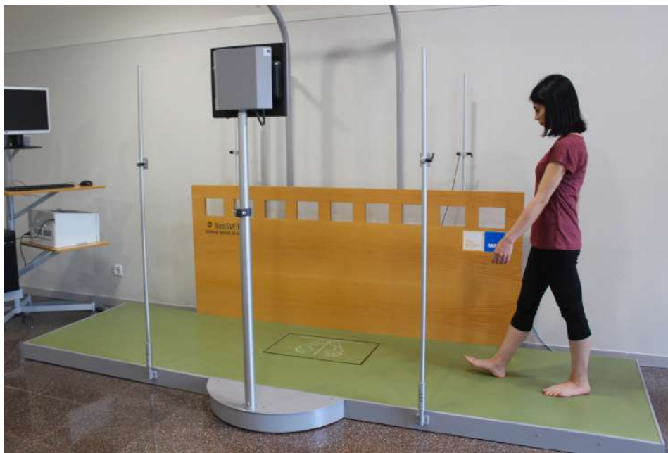
Figure 5.15: NedAMH/IBV ® gait analysis system that allows the integration of gait and balance analysis.
