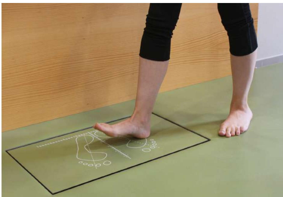
Figure 5.16: Detail of the dynamometric platform used for gait assessment. Participants walked repeatedly while stepping on the dynamometric platform.
