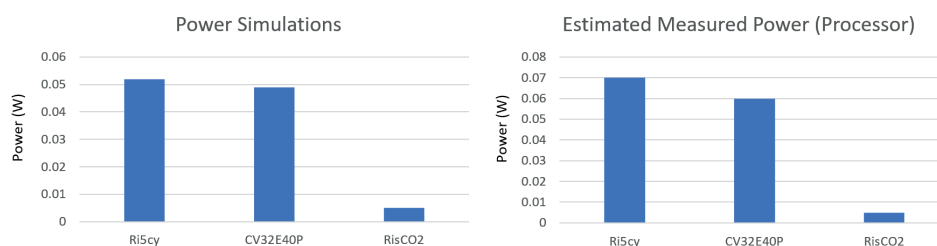
Figure 4.8: Comparison of simulated processor power consumption from Vivado with estimated power measurements inferred from Vitis.
