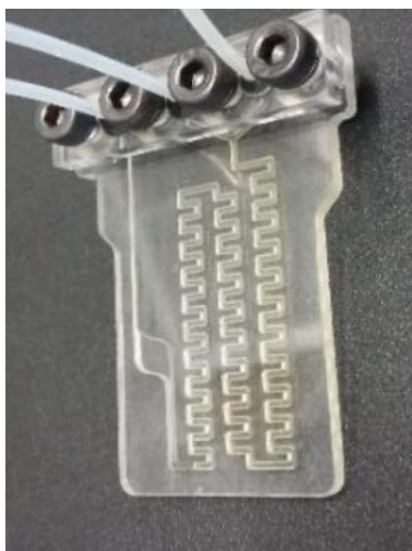
Figure 3.8: COC microfluidic platform with the tubing connected
