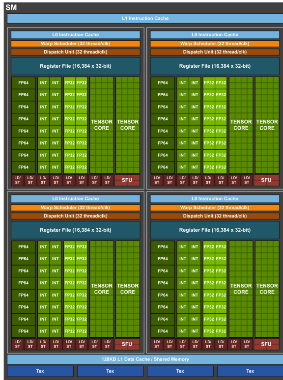
Figure 2.3: NVIDIA Volta GV100 Streaming Multiprocessor (SM); taken from Fig. 5 in [28]
