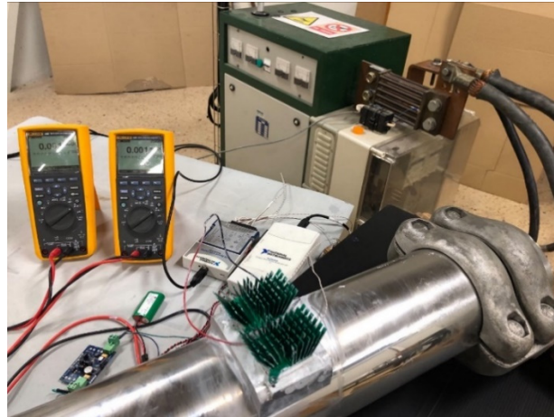
Figure 7. Experimental setup to characterize the performance of TEG #1 + DC/DC converter #1 mounted on a tubular conductor.
