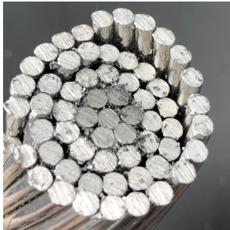
Figure 4-1. Cross section of a three-layer ACSR conductor.
