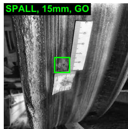
Figure 12. Picture of a mild spall defect.
