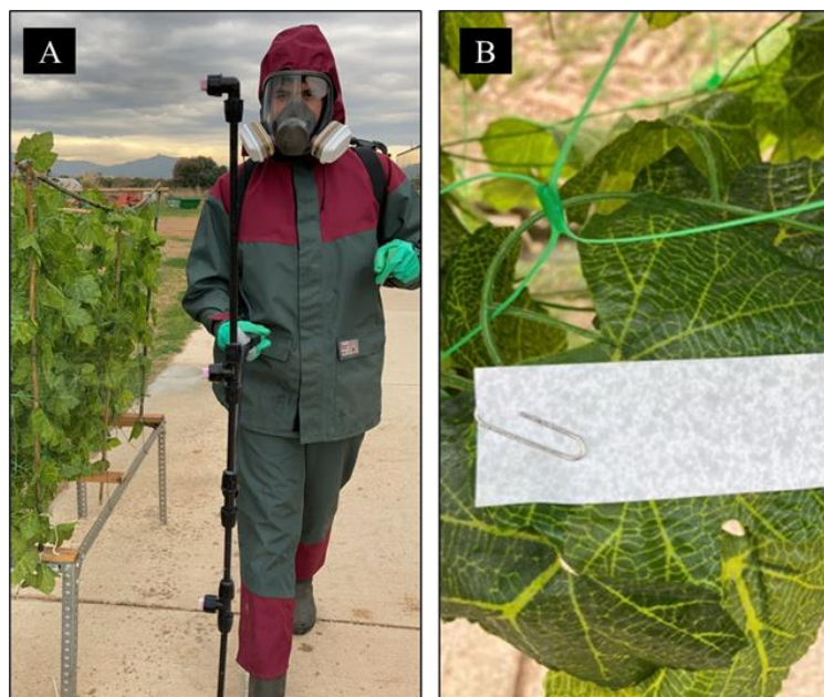
Figure 4.2. A: Spray application performance. B: Close view of the artificial collectors at the artificial vegetation.
