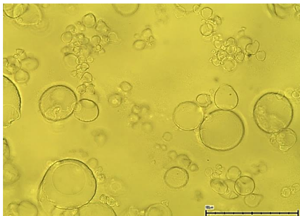
Figure 4.5. Optical microscope micrograph of wet microcapsules maturated in \text{CuSO}_4 aqueous solutions.
