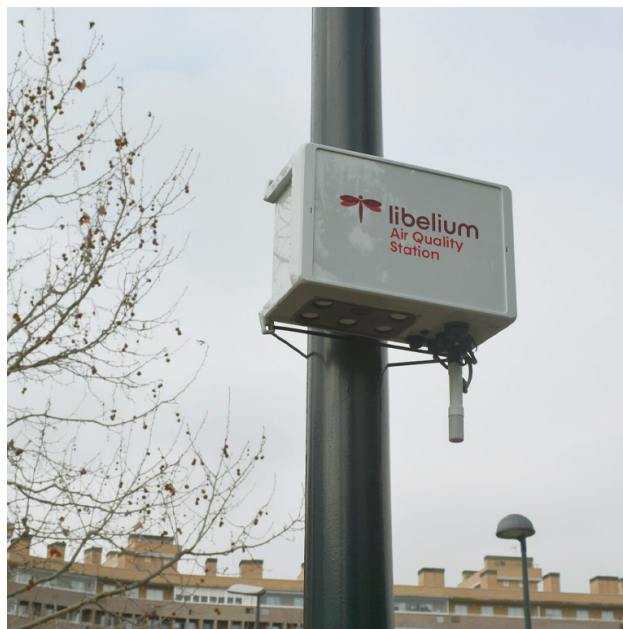
Figure 9: Libelium Air Quality Station installed on a pole. Extracted from libelium.com
