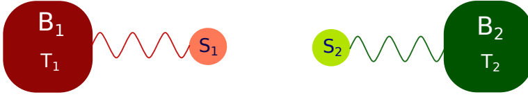
Figure A.1: A schematic of a situation where system S_1 is (semi-locally) interacting with the bath B_1 , and the system S_2 is semi-locally interacting with the bath B_2 . Temperatures of the baths are T_1 = \frac{1}{\beta_1} and T_2 = \frac{1}{\beta_2} .
