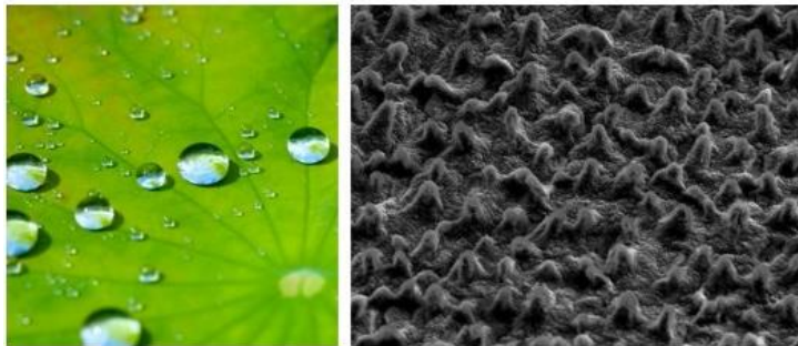
Figure 1.7 (Left) Photograph of a lotus leaf showing superhydrophobic behaviour. (Right) Scanning electron microscope image of the rough surface of a lotus leaf at the micro-scale 53 .
