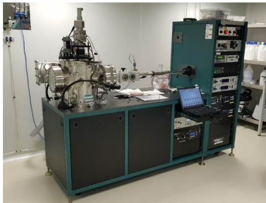
Figure 2.2 AJA Orion 8 HV Magnetron Sputtering System installed in the NanoFabrication laboratory at ICFO.
