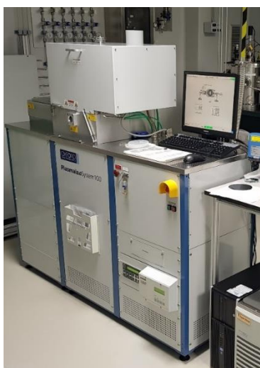
Figure 2.7 Plasmalab System 100 reactive ion etching system installed in the NanoFabrication laboratory at ICFO.
