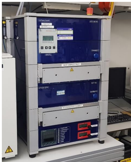
Figure 2.4 RTP-100-HV rapid thermal annealing oven installed in the Post-Processing laboratory at ICFO.
