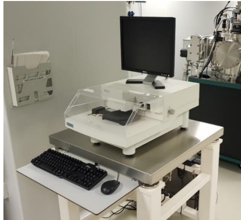
Figure 2.14 Tencor Stylus Alpha-Step profilometer from KLA installed in the NanoFabrication laboratory at ICFO
