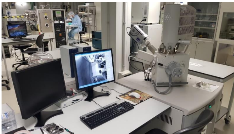
Figure 9 Scanning electron microscope Inspect F from FEI installed in the NanoFabrication laboratory at ICFO
