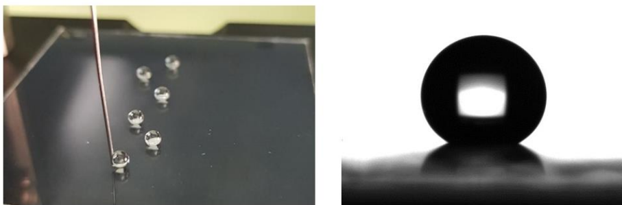
Figure 3.19 The water contact angle (CA) measurements were performed with a drop shape analyser, where multiple droplets with the same volume could be deposited in a controlled manner on the sample's surface (a). Image of a droplet of 7ul used to calculate the static CA (b).
