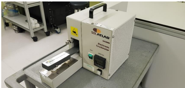
Figure 2.16 M238BB crockmeter installed in the Corning laboratory.
