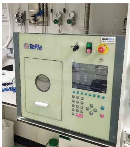
Figure 2.8 PVA TePla 300 SemiAuto plasma cleaner installed in the NanoFabrication laboratory at ICFO.
