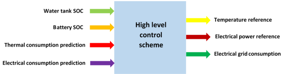
Figure 2.5: Control scheme for the CHP system
