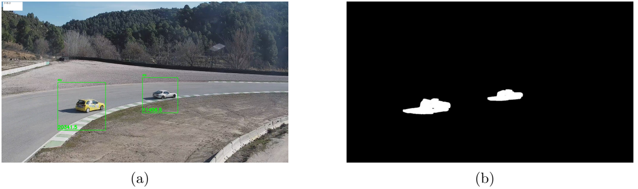
Figure 4.7: (a) Two cars in the racetrack with bounding boxes around them, obtained after performing background subtraction on the frame. (b) Thanks to a static background, the task of separating moving objects from the background is largely simplified. The regions of interest after applying simple computer vision techniques are much smaller than the whole FullHD frame captured by the camera lens, which allows us to focus the attention closer to the objects and increase the accuracy of the ground-truth model. In a scenario like the racetrack of the image, motion detection alone is able to filter all empty frames out and only consider those with cars and minimize the annotation costs.
