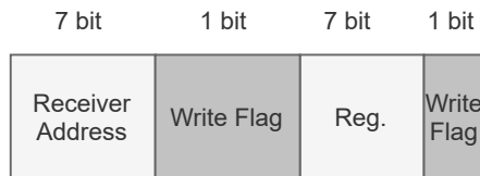
Figure C.2: I2C frame to perform register selection.
