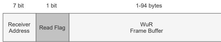
Figure C.5: I2C frame to read WuR-CTC frame buffer.
