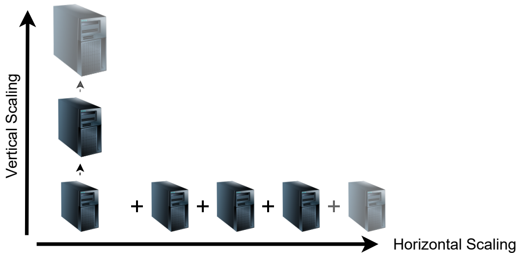
Figure 5.2: Vertical and horizontal scaling representation. The vertical axis represents the hardware upgrade or replacement, while the horizontal one represents the addition of further machines.
