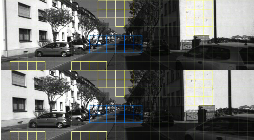
Figure 6.2: The figure compares two consecutive KITTI frames and highlights regions that exhibit spatio-temporal similarity. Yellow regions represent areas with low 2D frequency and high similarity. The blue regions correspond to distant areas in the scene that move slowly due to parallax.
