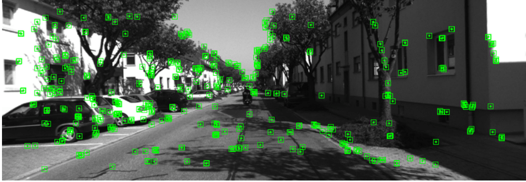
Figure 2.6: Illustration of ORB feature extraction on a KITTI dataset image, with green points marking the detected features.
