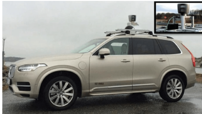
Figure 3.2 A LiDAR mounted on a vehicle. The sensor is typically placed on top of the vehicle to avoid occlusion and exploit its full range of operation. Adapted from [154].
