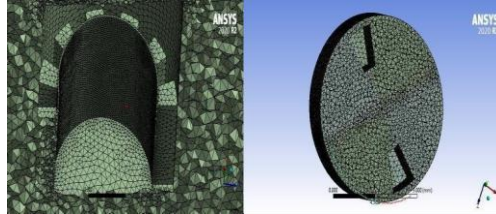
Figure 2.6 Tetrahedral mesh of (a) stator and (b) rotor
