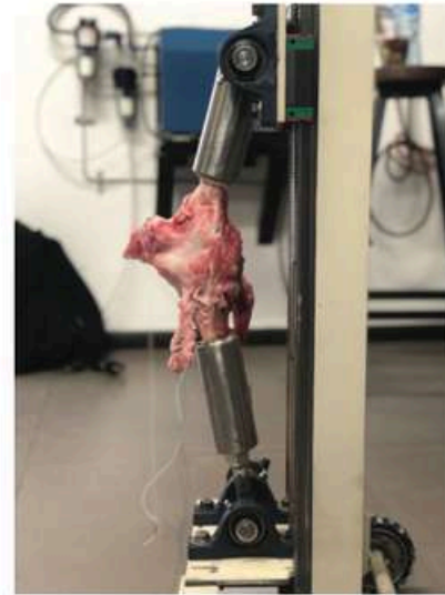
Figure 3. Custom-made testing apparatus. Medial view of a porcine right knee showing the preparation of the muscle groups.
