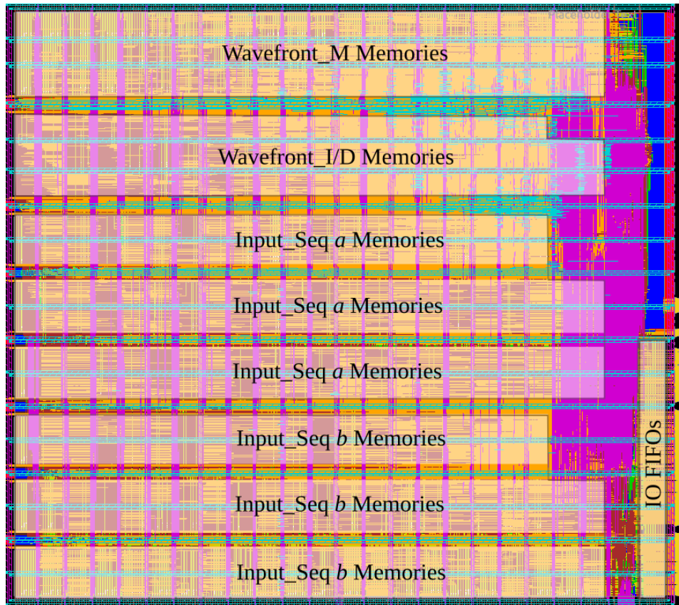
Figure 6.4: Accelerator layout. The size is 1330\mu\text{m} \times 1200\mu\text{m} with all the connectivity on the right side.
