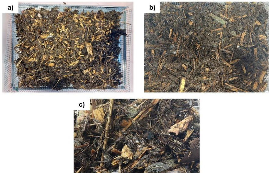
Figure 6.2 SSF in tray bioreactor. a) Initial material of the fermentation, b) Fermented material after 10 days of process, c) Fermented material from a closer view to observe Trichoderma .
