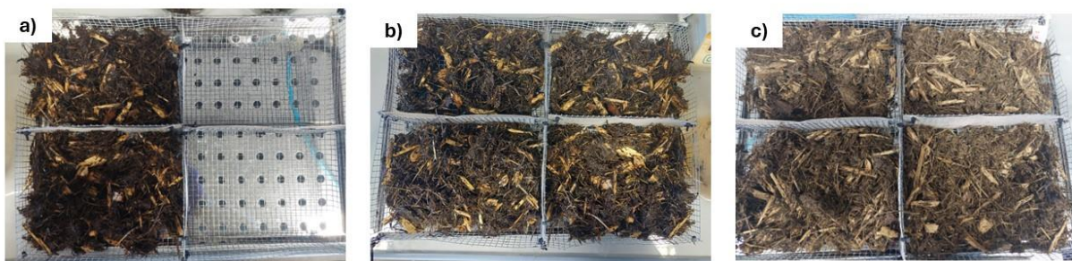
Figure 6.11 Performing SSF in one tray with conditions. a) SSF with 0.2% Trp, b) SSF with 0.2% (left) and 0.43 (right) % Trp, c) Final appearance of SSF tray reactor.
