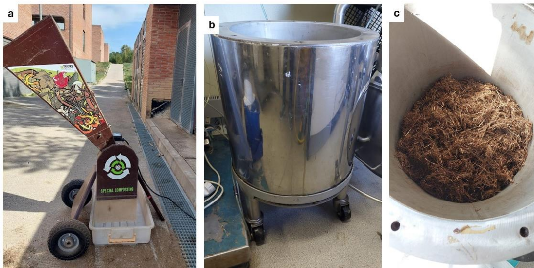
Figure 3.2 a) The compost shredder used to chop the grass clipping; b,c) air drying the grass in a biodrying reactor
