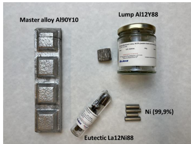
Figure 15. Raw materials used for the preparation of Al 86 Ni 8 Y 4,5 La 1,5 alloy.
