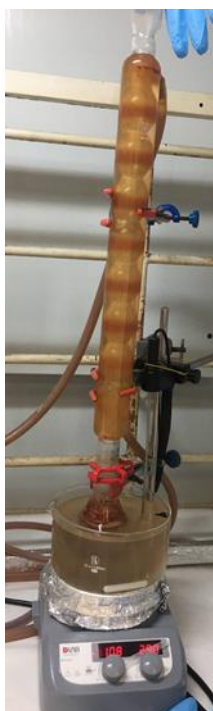
Figure III.15. Digital photograph of reaction setup of cork/glyphosate in toluene at 120 °C.
