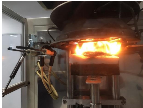
Figure III.33. Digital photograph of cone calorimeter while burning a sample.
