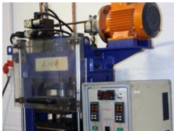
Figure III.19. Digital photograph of the hot-plate press.
