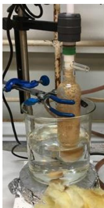
Figure III.14. Digital photograph of reaction setup of cork/glyphosate in water at 120 °C.
