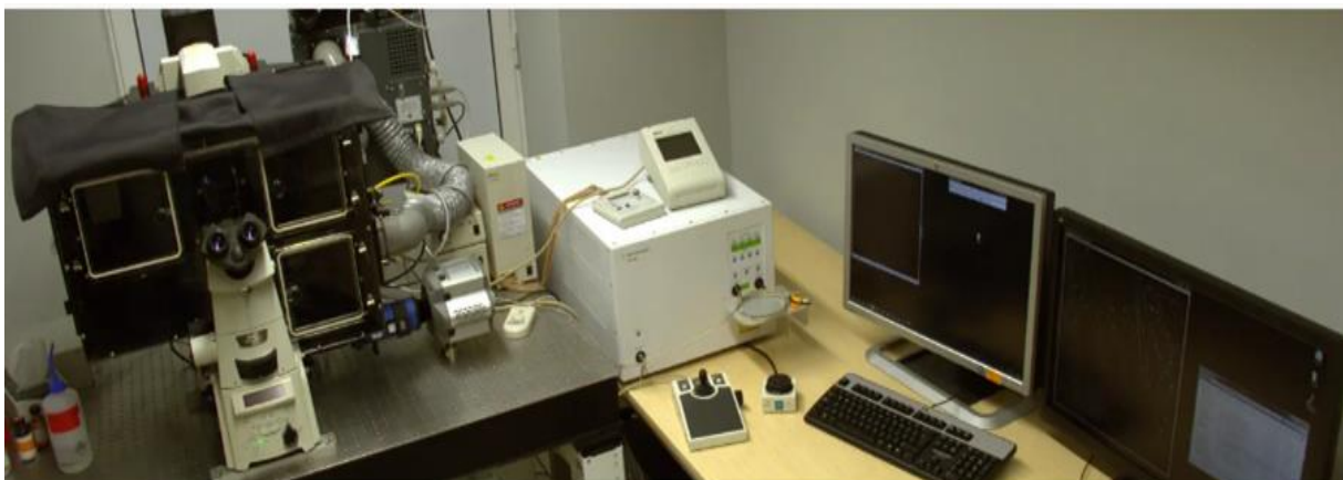
Figure 1.10. Nikon inverted fluorescence microscope (Nikon Eclipse Ti) in the NSTORM laboratory of the super-resolution and nanoscopy laboratory at ICFO.
