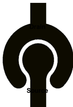
Figure 5.2. Corbino layout with a channel length equal to 20 nm.
