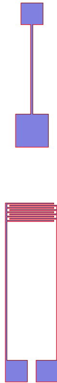
Figure S1. Device layout. W=18000\ \mu\text{m} , L= 50\ \mu\text{m} , W/L=360 . The coplanar gate electrode's area is equal to 2.25\ \text{mm}^2 .
