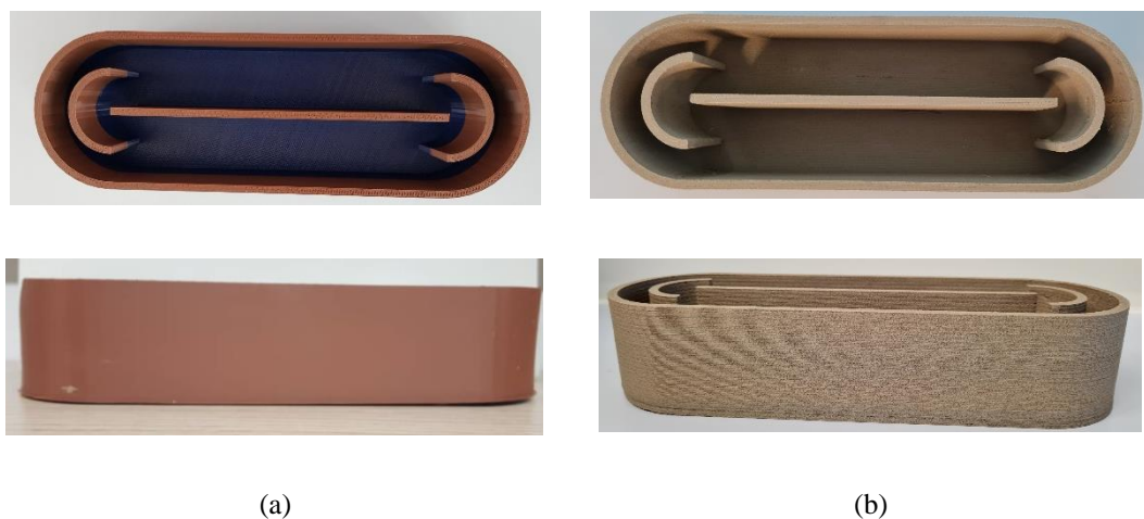
Figure 8-6 Image of the 3D-printed Race Pond Reactors (RPRs): PLA (a) and Timberfill® (b)
