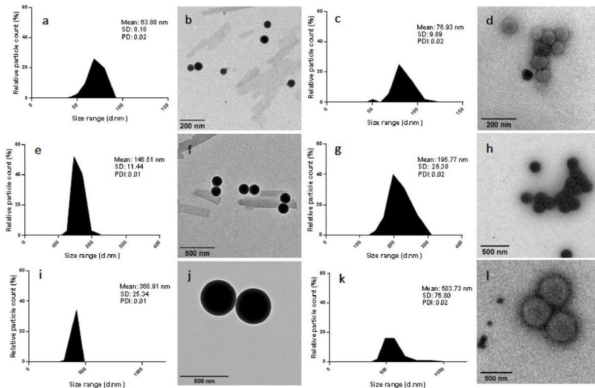
**Fig. 1.** The graphs indicate the size distribution (mean ± SD) and polydispersity index in water and in supplemented RPMI-1640, of PS-50 (a, c); PS-200 (e, g); and PS-500 (i, k). The TEM images show round shapes in both water and in supplemented RPMI-1640 for PS-50 (b, d), PS-200 (f, h), and PS-500 (j, l).
