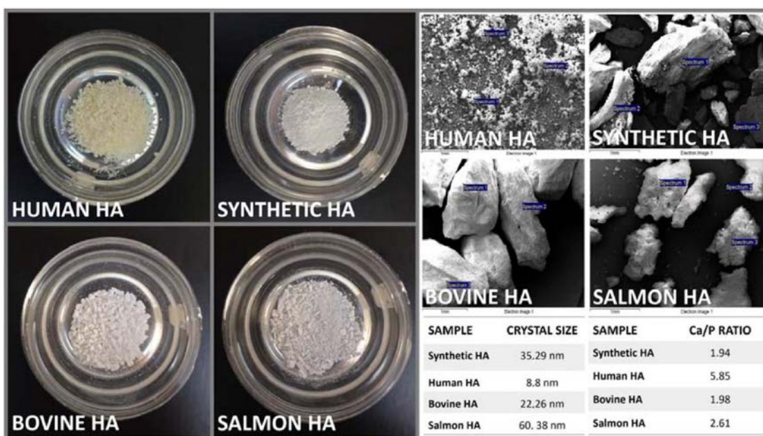
Figure 1. Prepared control and experimental HA samples (Left) before characterization and analysis. SEM micrographs of control and experimental HA samples (Top Right). Crystal size control and experimental HA samples obtained via XRD and the Ca/P ratio (atomic weight %) for control and experimental HA samples obtained via SEM/EDS (Bottom Right). The crystal size, studied using XRD and further analyzed using the Scherrer equation, reported sizes ranging from 8.8 nm to 60.38 nm. Using SEM/EDS analysis, the Ca/P ratio (atomic weight %) for the samples determined the lowest values for our salmon HA and bovine HA with 1.94 and 1.98, respectively, yet these were similar/close to what is often presented in the literature ( the theoretically stoichiometric value of HA was set at 1.67 ), validating our experimental protocol. It is noteworthy that all other HA yielded values higher than those commonly reported in the literature. The Ca/P ratio (calcium-to-phosphorus ratio) in terms of the atomic weight percentage (%) is calculated by dividing the atomic weight % of calcium (Ca) by the atomic weight % of phosphorus (P). The atomic weights of Ca and P are approximately 40.08 g/mol and 30.97 g/mol, respectively. As mentioned, human HA has a Ca/P ratio close to 1.67 in its ideal form. Any deviations from this ratio can indicate changes in the bone mineral density and quality.
