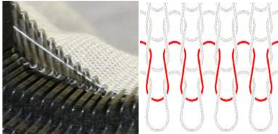
Figure 39. Knitting process and schematic of the loops.
