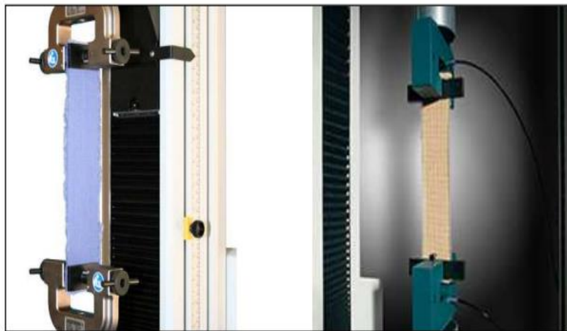
Figure 52. Strip method test. Sources: Left Instron. Right: Vidal protection [97].
