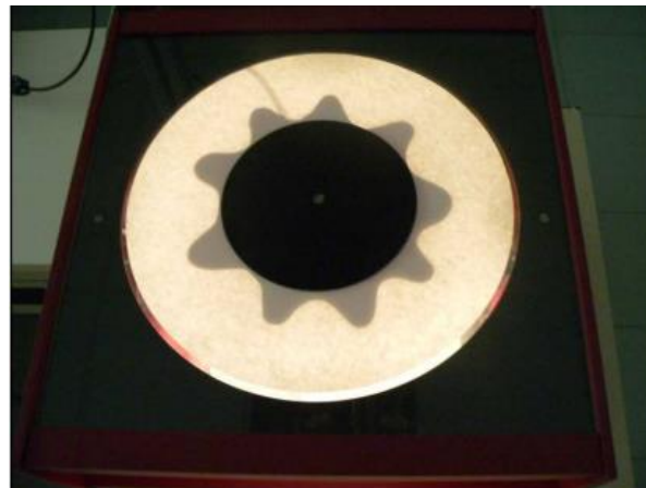
Figure 61. The profile of the cast shadow of the fabric falls on a Cusick drosometer [97].
