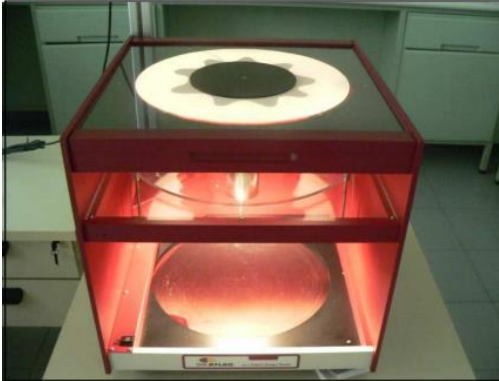
Figure 59. Top view of the current version of the Cusick diameter marketed by the SDL Atlas. Fountain [97].
