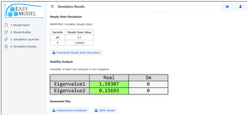
Figure 5.12: Steady State Simulation results: Unstable steady state is found. Stability analysis delves in the analysis by displaying the Eigenvalues. Results are in accordance with COPASI's (see Figure 5.1).
