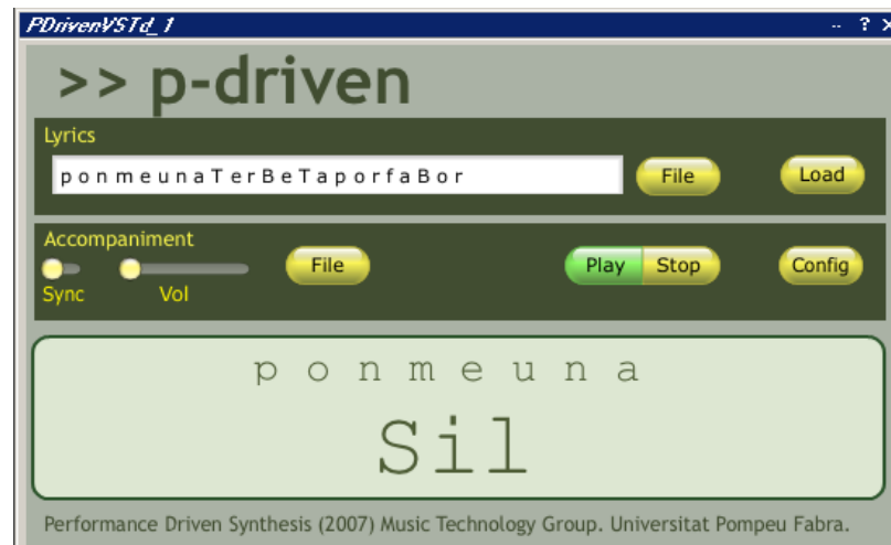
Figure 4.13: Screen-shot of the PDriven prototype. Users can type or load a text file with the lyrics in SAMPA format. In karaoke-like situations it can be supported with accompaniment music.
