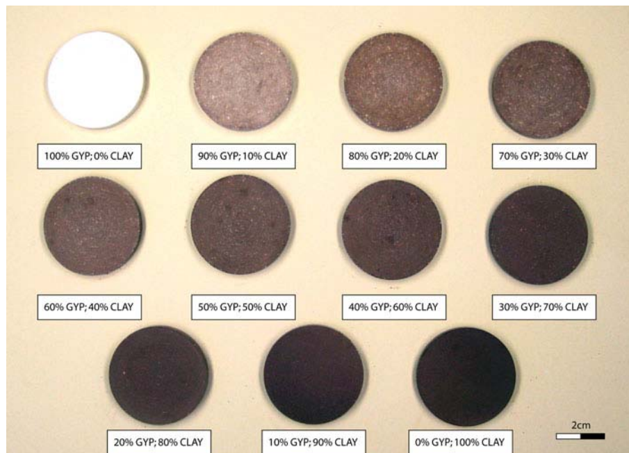
Fig. 3 Sample pills made using mixtures of powdered clays and \text{CaSO}_4 \cdot 2\text{H}_2\text{O} laboratory reagent in different proportions (100–0% gypsum contents in intervals of 10%)
