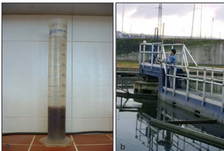
Figure 3.6 Sludge settleability measurements: (a) V30 test and (b) sludge blanket measurement
