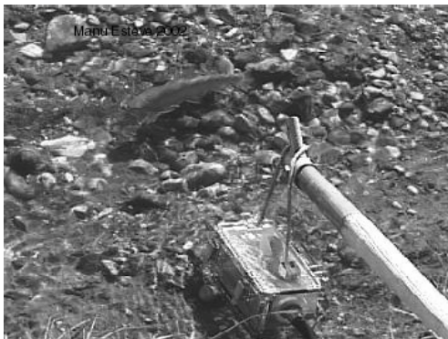
Figure 1. A camera inside an acrylic housing attached to a rope records a brook trout female on a redd.
