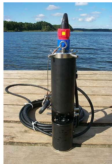
Figure 3.7 (Left) Chlorophyll measuring device (Fluoroprobe, BBE, Inc.) (Right) Fluoroprobe 's light sources emitting at selected wavelengths.
