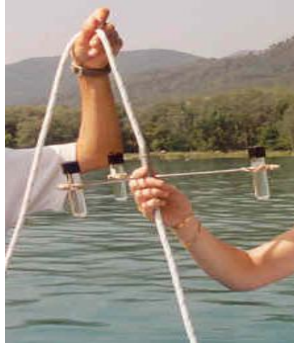
Figure 3.9 Sediment tramps arrays. It has place for 6 bottles although they are only three used in the photo.
