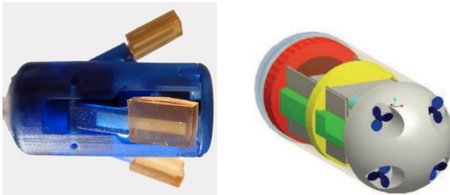
Figure 3.3: Overall design of the actuation system for the locomotion in the esophagus and in the stomach respectively. Images taken from [17] and [18].
