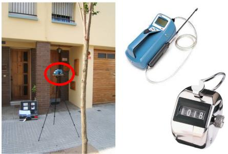
**Figure 10.** Picture of the mobile condensation particle counter (P-Trak) and tally counter and setting used to monitor outdoors of participants' homes.
