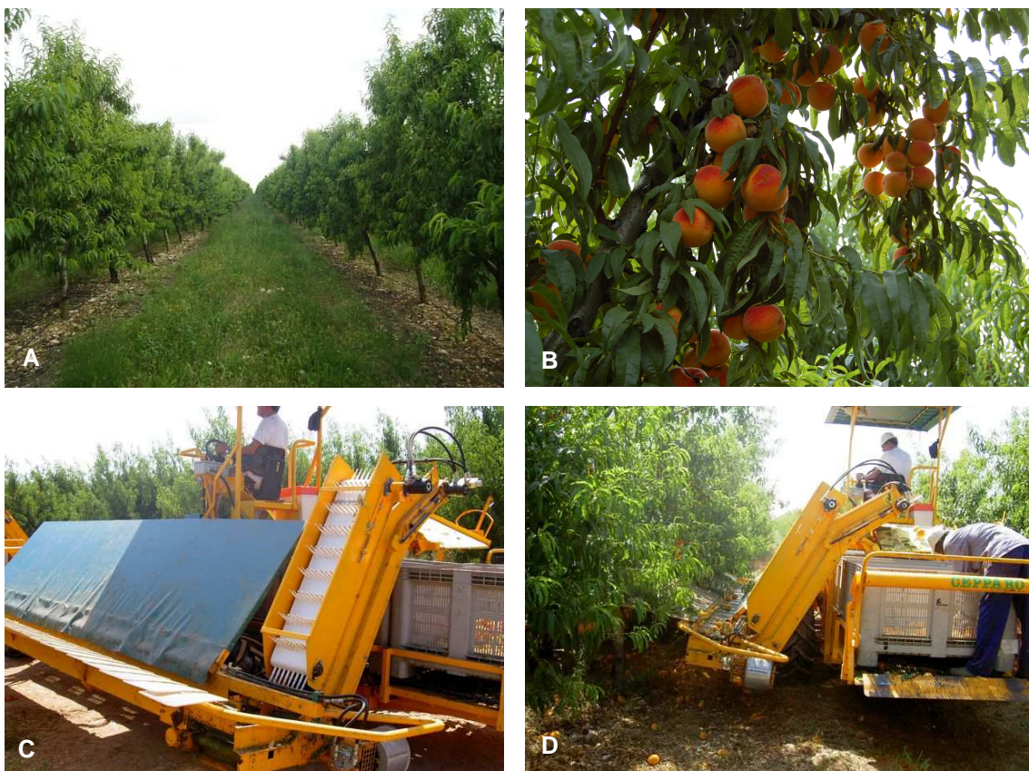
Figure 6. Peach orchard at mid May (A), fruit of cv. Andross (B) and mechanical harvesting with a continuum trunk shaker (C and D).
