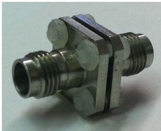
Figure 2.8: Experimental sample assembly for MW measurements on a thin TiN film.
