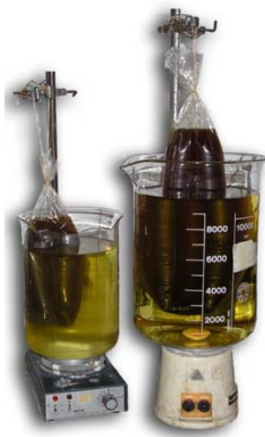
Figure 2.8. Dialysis process used for purification of xylo-oligosaccharides.
