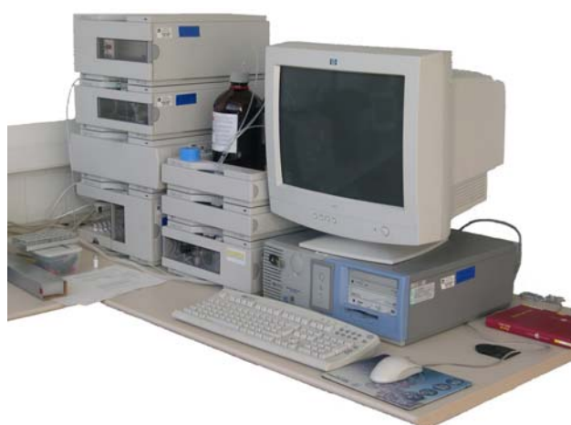
Figure 2.9. Equipment used for HPLC/GPC.
