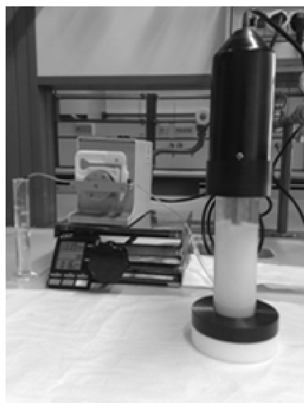
Figure 3.4. Stirred cell emulsification set-up
